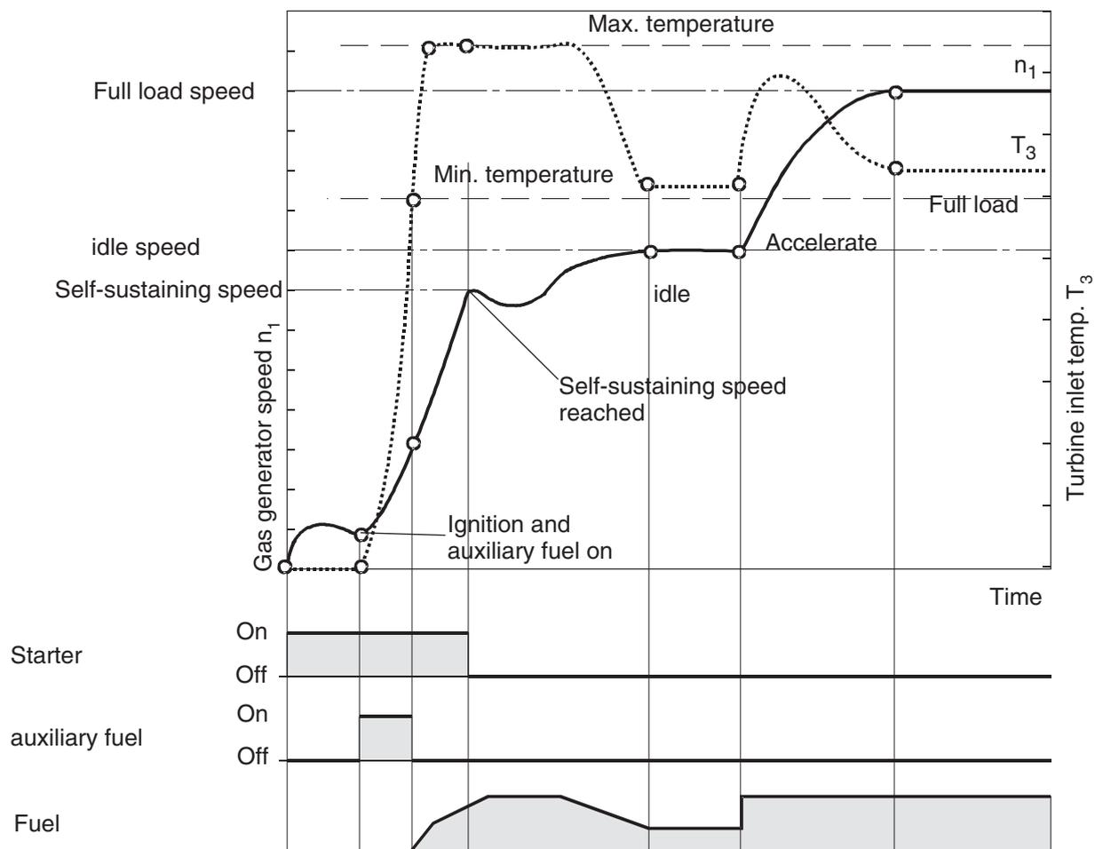
Fig. 2.10 Start-up procedure
