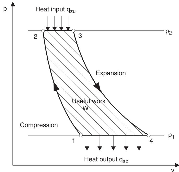
Fig. 4.3 p/v diagram of gas turbine process
