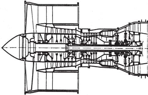
Fig. 1.1 Jet engine for the propulsion of an aircraft
