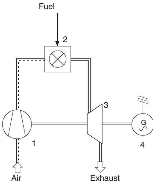
Fig. 4.1 Simple, open gas turbine system
