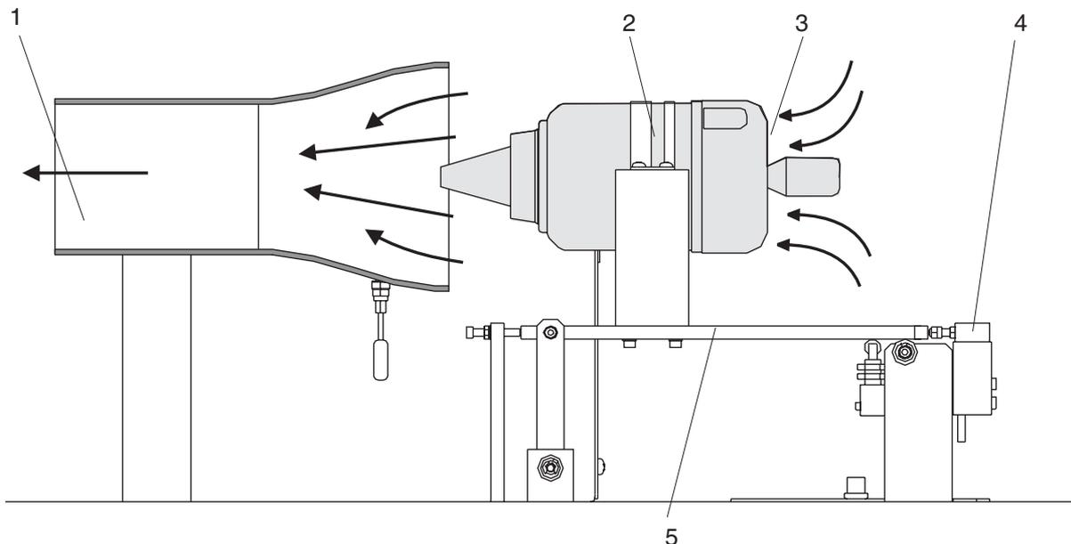
Fig. 2.4 Jet turbine with mixing tube and thrust measurement
