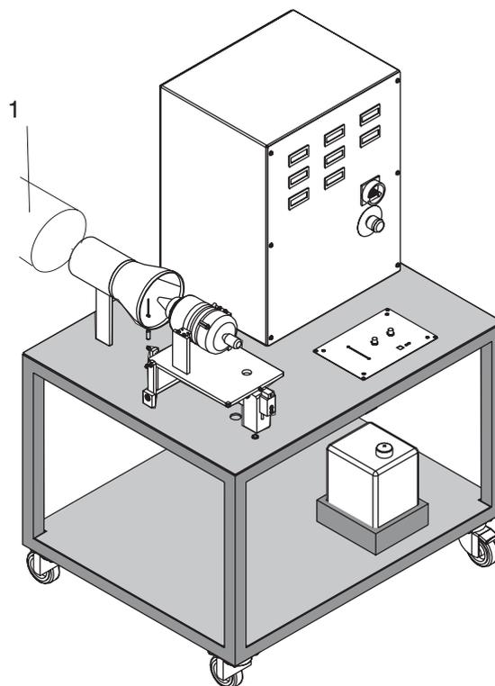
Fig. 2.8 Turbine with exhaust pipe (1)
