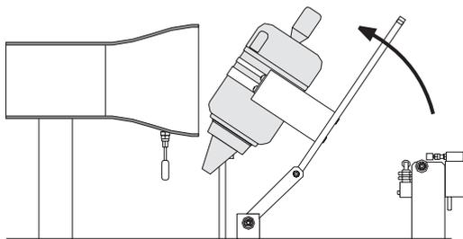
Fig. 2.11 Swivel turbine to remove residual fuel
