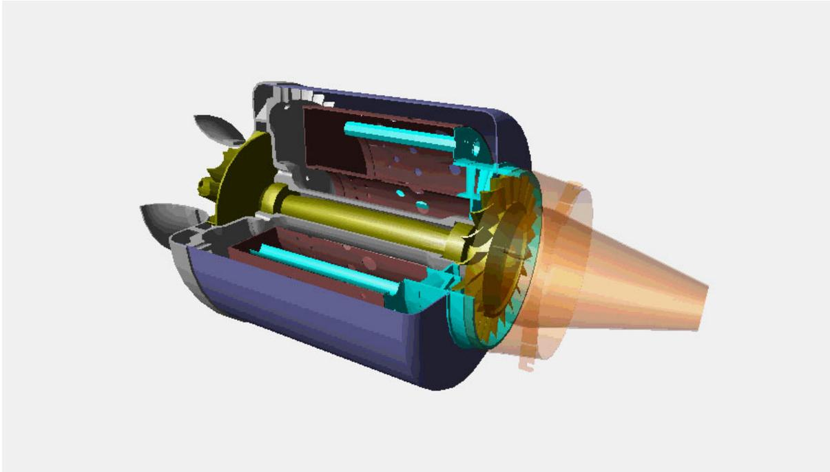
Fig. 2.2 Model jet turbine
