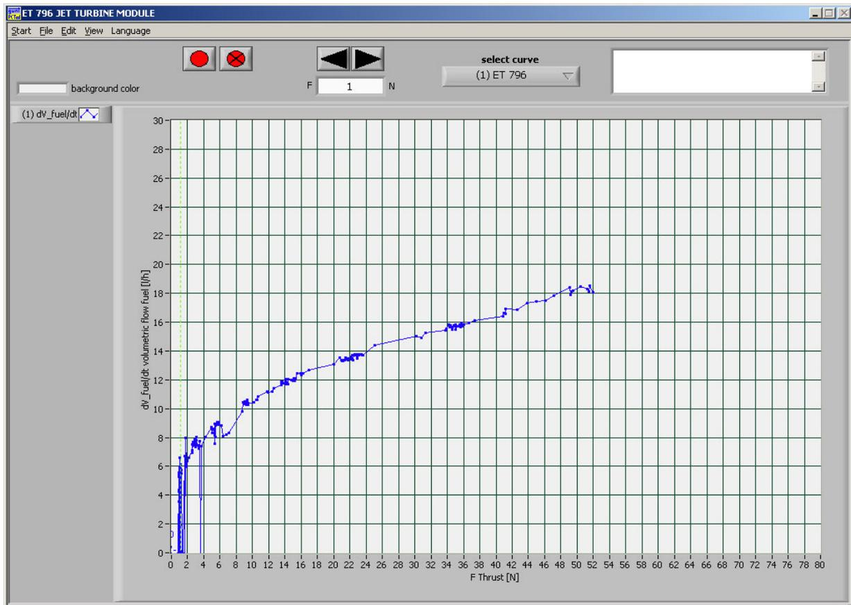
Fig. 5.3 Fuel-consumption dependance on thrust
