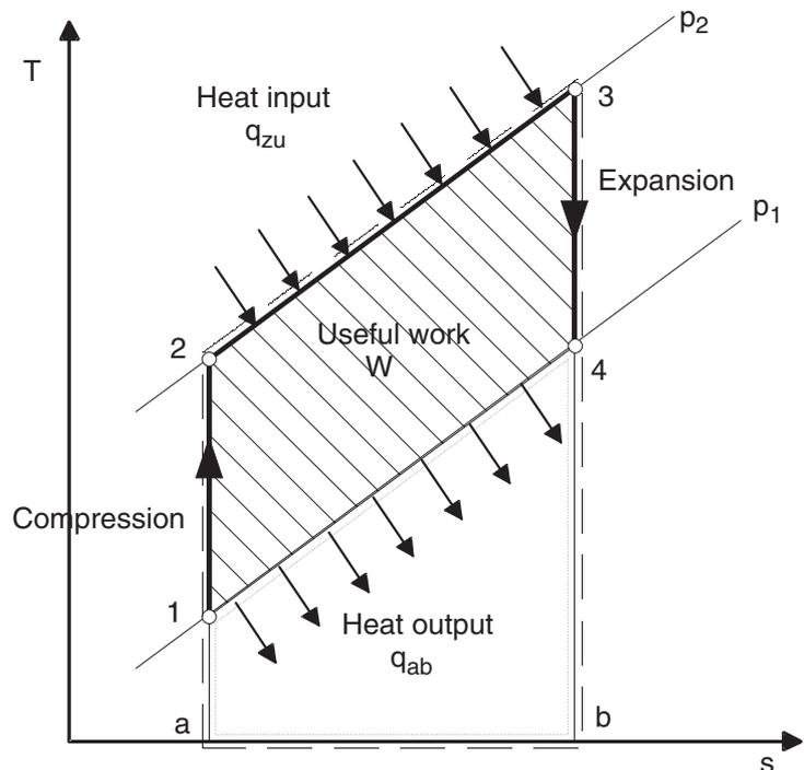
Fig. 4.2 T,s-diagram of gas turbine process
