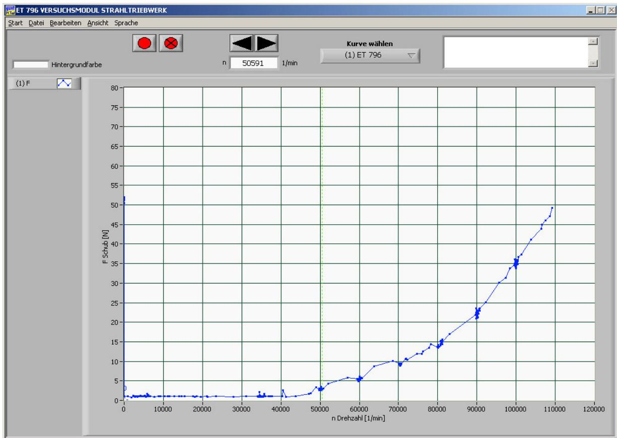
Fig. 5.2 Thrust of the jet turbine from start up to 120000 rpm.
