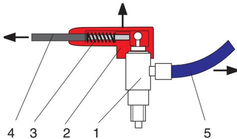
Fig. 2.12 Glow plug connection
