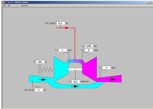
Fig. 5.1 System diagram of a gas turbine
