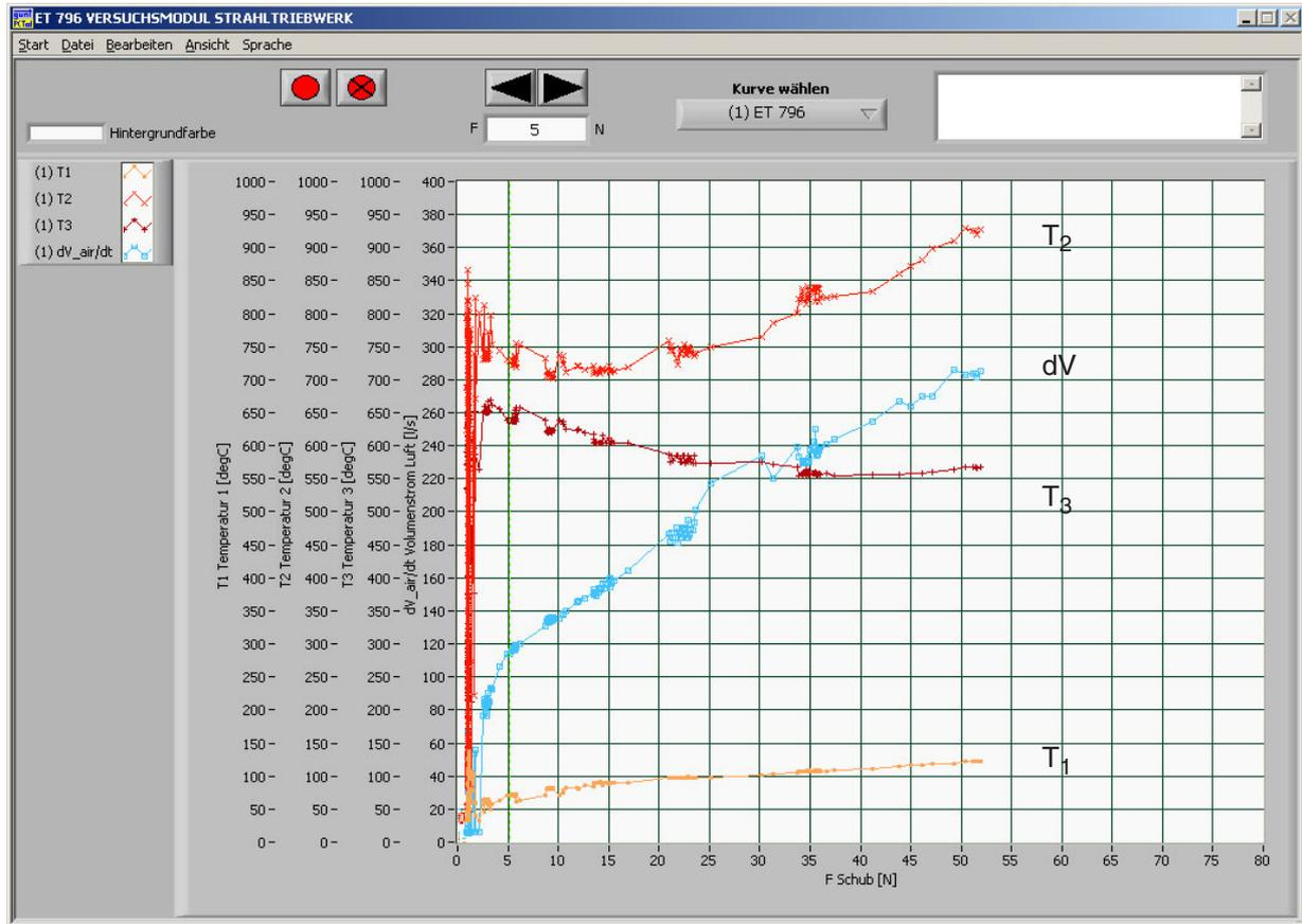
Fig. 5.4 Temperatures and air consumption of the jet turbine dependent on thrust
