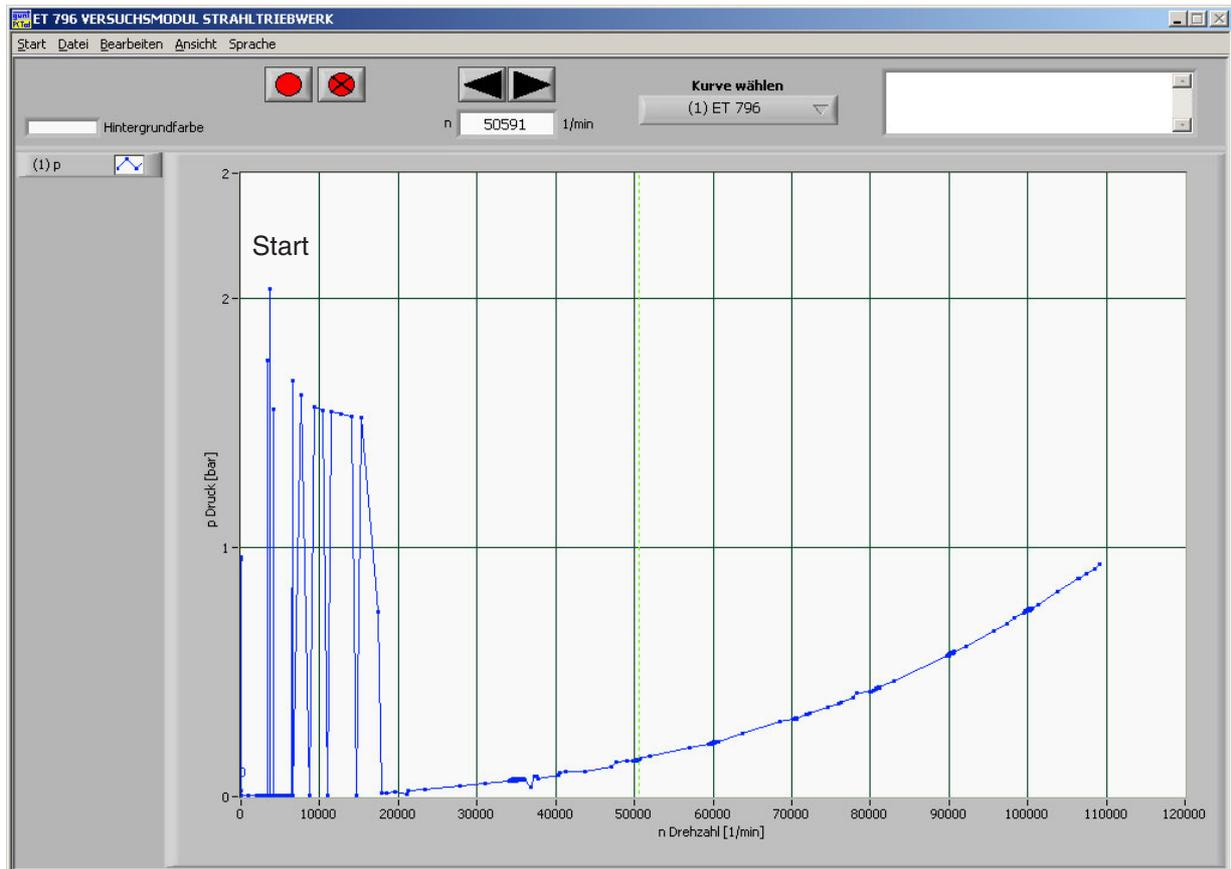
Fig. 5.5 Combustion chamber pressure of the jet turbine from start up to 120000 rpm.
