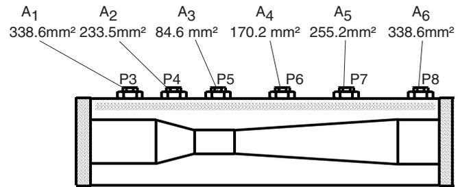
Fig. 6.17 Venturi nozzle with rectangular tube section
