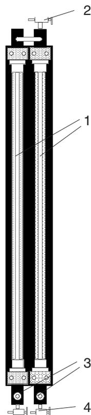
Fig. 5.1 Two tube manometer
