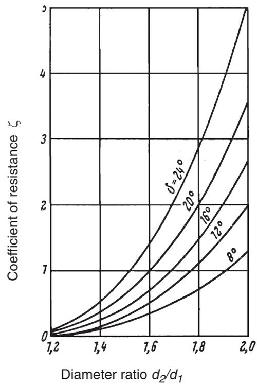
Fig. 7.5 Coefficients of resistance for continuous expansion (diffusor) as a function of contraction angle  $\delta$
