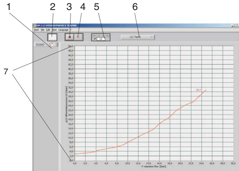
Fig. 4.2 "Measurement diagram" window
