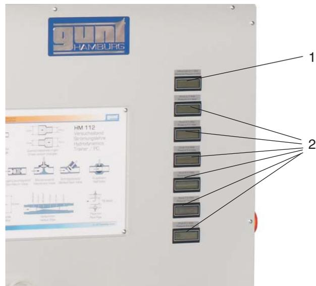
Fig. 2.5     Switch cabinet with digital displays
