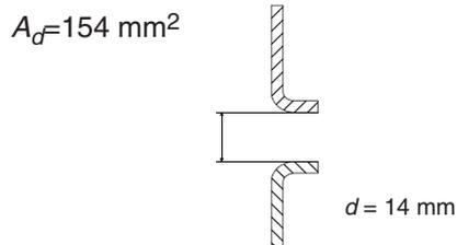
Fig. 6.15 Nozzle cross-section
