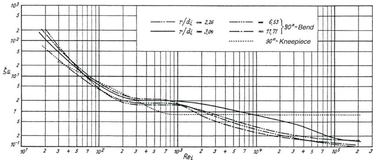
Fig. 6.3 Coefficients of resistance of smooth 90° elbows (VDI Wärmeatlas 10. Aufl. 2006)
