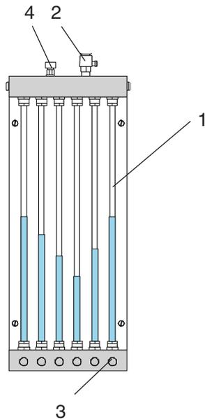
The six tube manometer comprises six glass level tubes (1) with a mm scale behind them.
