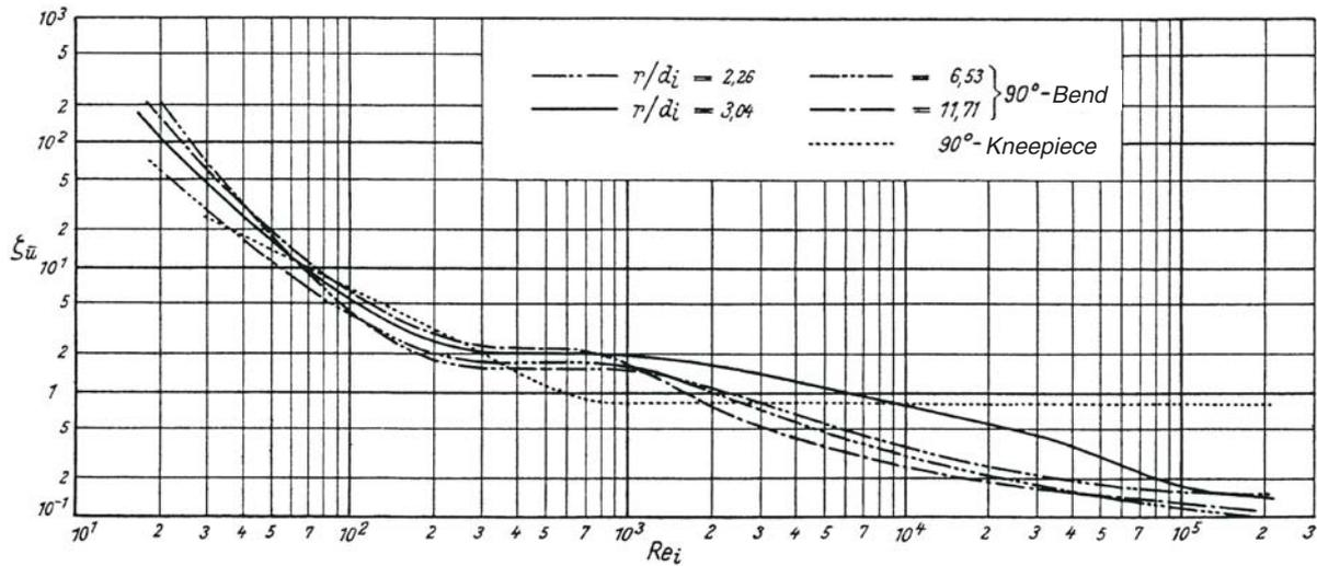
Fig. 7.2 Coefficients of resistance of smooth 90° elbows (from VDI Wärmeatlas 10. Aufl. 2006)
