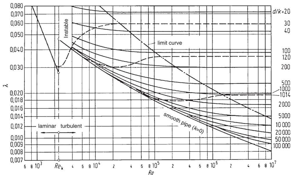
Fig. 6.1 Pipe friction coefficient corresponding to Colebrook and Nikuradse (taken from "Dubbel: Taschenbuch für den Maschinenbau") [Engineering Handbook]
