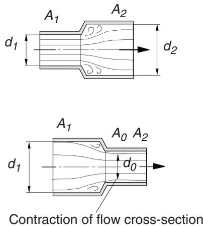
Fig. 6.4 Change of cross-section
