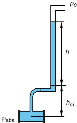
Fig. 5.3 Absolute pressure measurement
