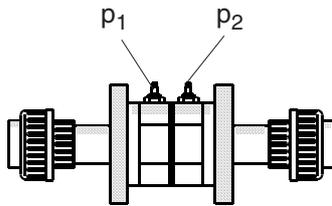
Fig. 6.13 Nozzle/orifice
