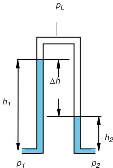
Fig. 5.2 Differential pressure measurement
