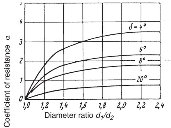
Fig. 7.4 Wall friction factor for continuous contraction (nozzle) as a function of contraction angle  $\delta$
