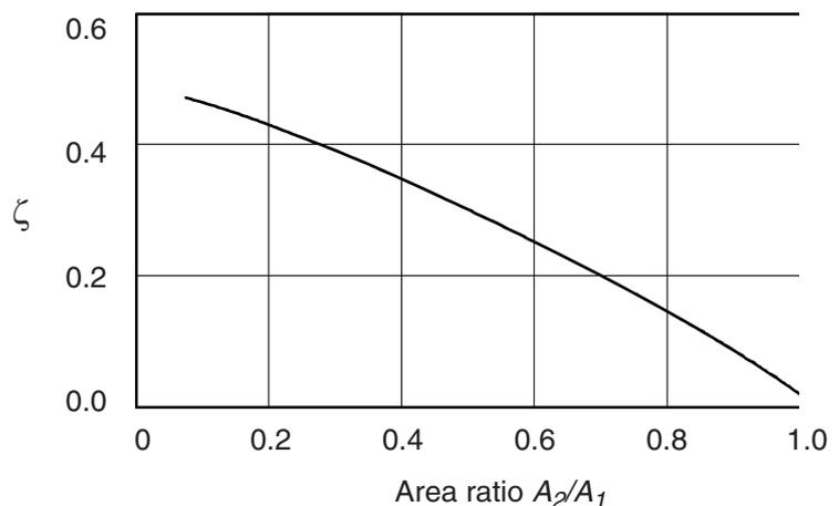
Fig. 6.5 Coefficient of resistance for discontinuous contraction
