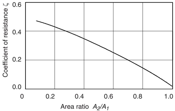
Fig. 7.3 Coefficient of resistance  $\zeta$  for discontinuous contraction
