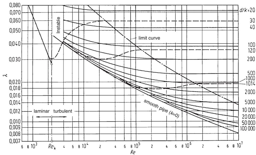
Fig. 7.1 Pipe friction coefficient corresponding to Colebrook and Nikuradse (taken from "Dubbel: Taschenbuch für den Maschinenbau") [Engineering Handbook]
