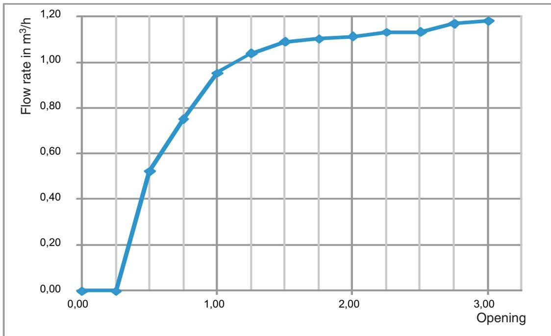
Fig. 6.11 Opening characteristics of valves
