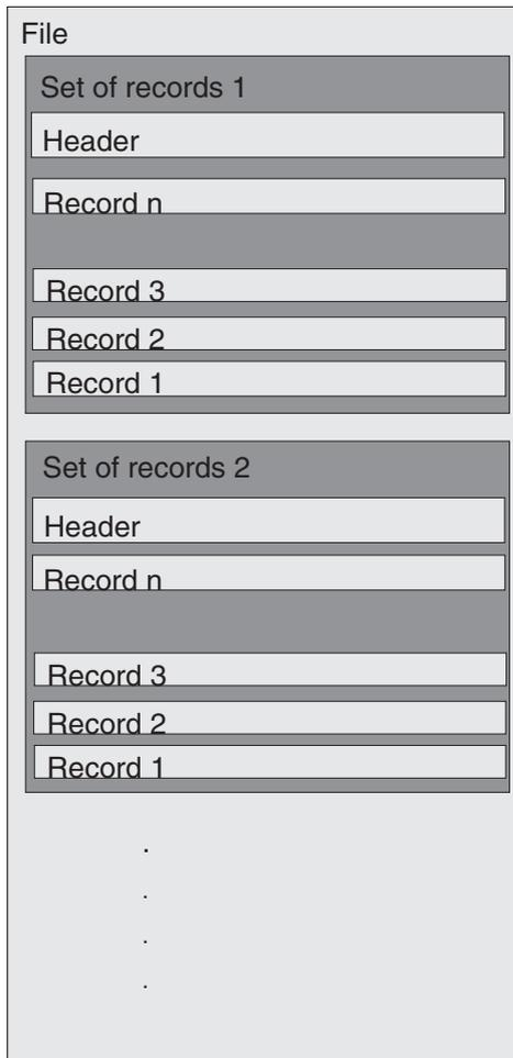
The measured data file can consist of several measuring series.
