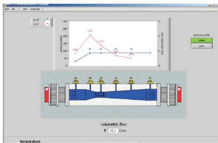
Fig. 4.3 “Venturi Nozzle” window
