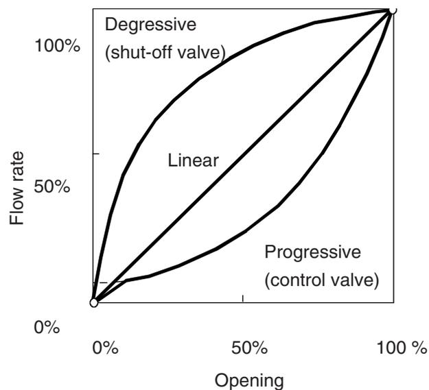
Fig. 6.10 Opening characteristics of valves
